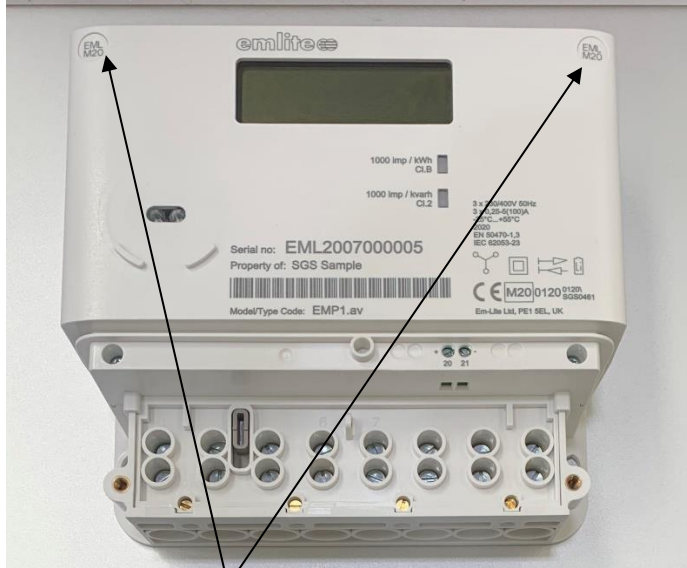
Main cover sealing
