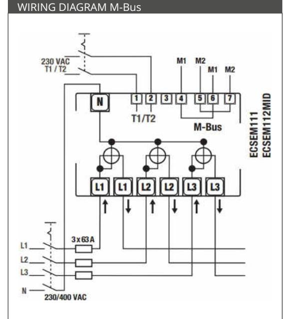
The connection of the neutral wire to the "N" terminal of the energy meter is mandatory.
