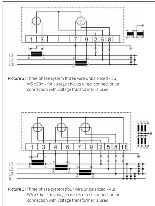
Picture 2: Three phase system (three wire unbalanced - 3u)
