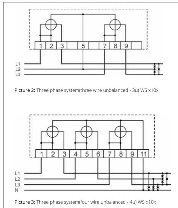
Picture 2: Three phase system(three wire unbalanced - 3u) WS x10x
