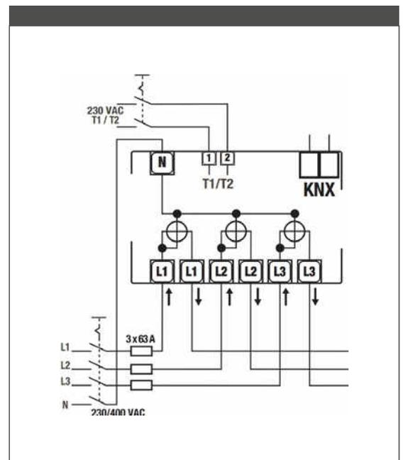
The connection of the neutral wire to the "N" terminal of the energy meter is mandatory.
