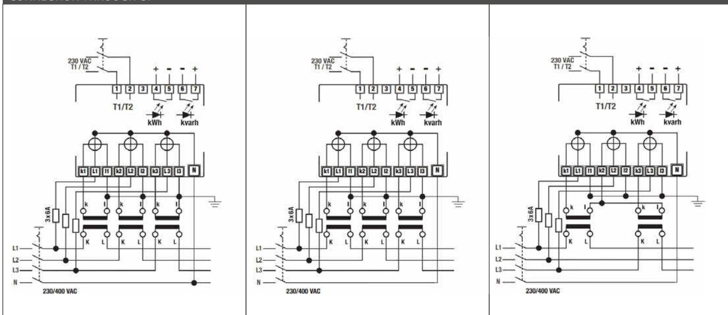
Neutral wire must be connected to the meter
